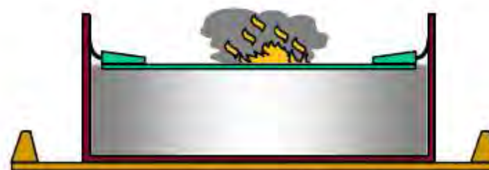
Spill on Roof Fire
